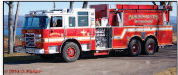
NEW ENGINE – MEREDITH 14E4A 2016 Pierce with Arrow XT chassis and Detroit Series 60 525 HP. Transmission: Allison Gen IV 4000 EVS 6 speed. Pump: Waterous 1,750 GPM. Tank: 2,500 Gallon. Foam: 20 Gallon Pierce Husky™ 3 Foam System. Ladders: 28' / 16' / 10' Ground Ladders. Deck Gun: Pre-piped deluge gun. Crew Capacity: 6. This truck also has a 2,500 gallon Folda-Tank and carries 1,200 feet of 5-inch supply hose.
