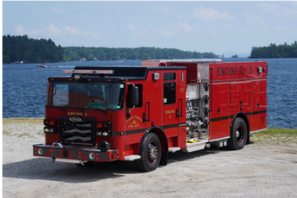
Center Harbor Enforcer Pumper Job #37096 1500gpm Pump / 1250 Gallon Tank
