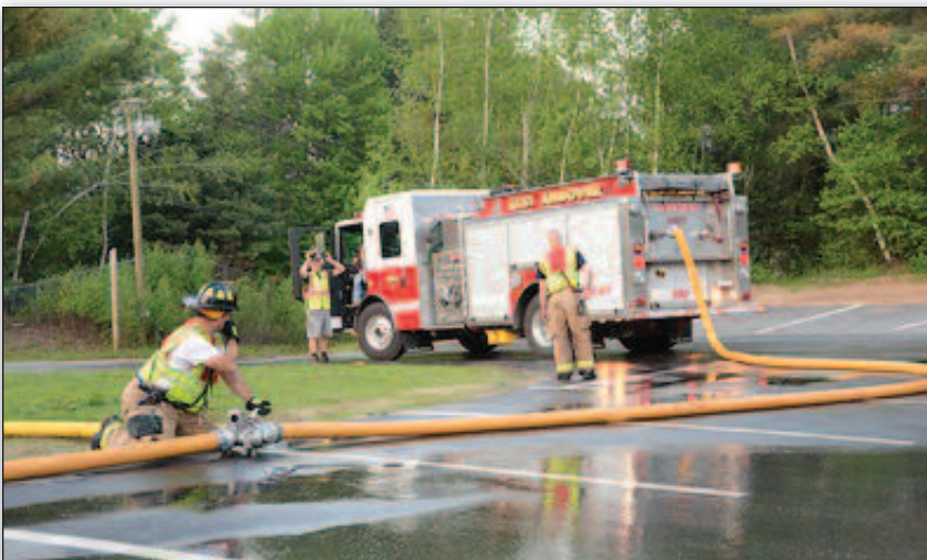
7E3 established a fill site designed to fill two tankers.
