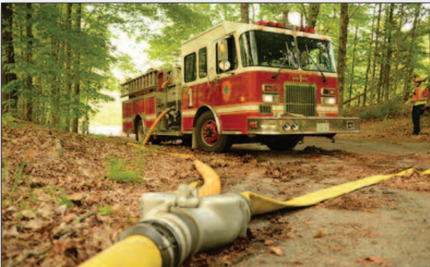
Rural Hitch established to allow two off load sites.
