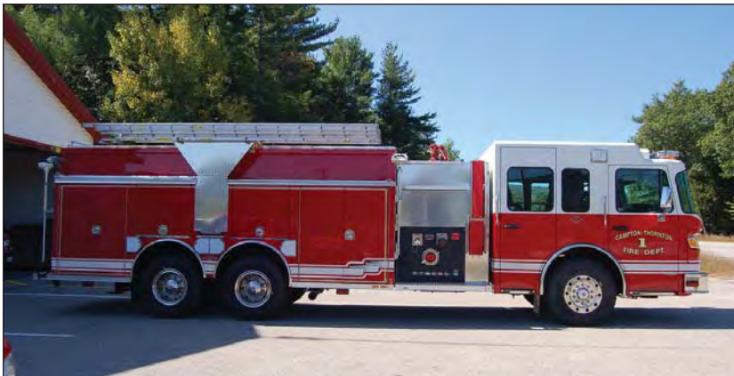
Campton-Thornton. 35Engine1 The truck was built by Rosenbauer on a Spartan Diamond chassis. It has a 1,500 GPM pump and a 2,500 gallon tank.
