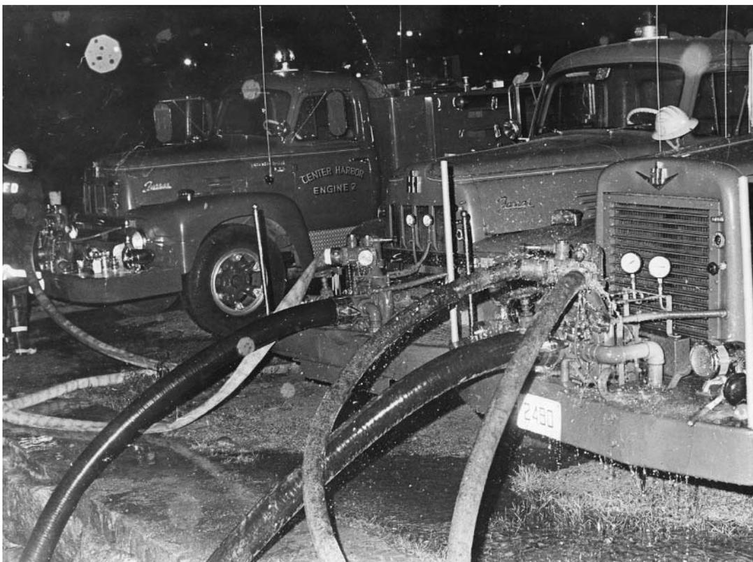
**Fire fighting apparatus circa 1950. Most trucks in this area were equipped by Farrar, a manufacturer of fire trucks in the forties and fifties. These used an International chassis.**
